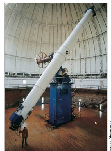
FIGURE 3-12 The Yerkes refractor, still one of the two largest in the world, has a 1-m-diameter lens.
